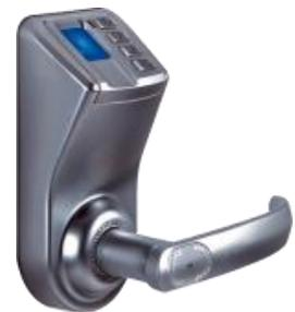
Figure 4. Fingerprint scanner.
